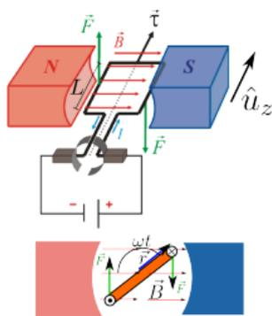
$$\begin{aligned}\vec{\tau} &= 2\vec{r} \times \vec{F} \\ &= 2riB|\sin(\omega t)|L\hat{u}_z\end{aligned}$$
