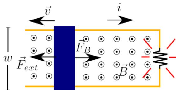
$$\begin{aligned}\mathcal{E} &= Bwv & i &= \frac{Bwv}{R} \\ |F_B| &= Biw = \frac{B^2w^2v}{R} \\ P_e &= i^2R = \frac{B^2w^2v^2}{R} \\ &= F_Bv = P_{mec}\end{aligned}$$
