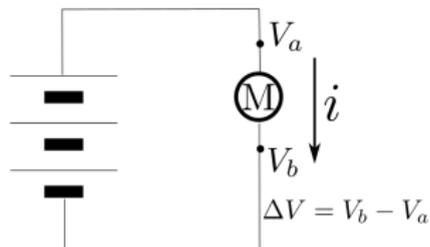
$$P_{\text{mec}} = Ni \left\| \frac{\partial \vec{S} \cdot \vec{B}}{\partial t} \right\|$$
