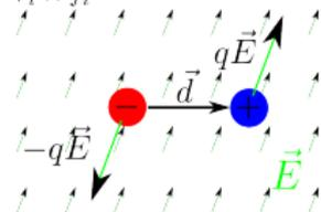
$$\begin{aligned} \sum_i \mathcal{T}_i &= \frac{\vec{d}}{2} \times (q\vec{E}) - \frac{\vec{d}}{2} \times (-q\vec{E}) \\ &= \vec{p} \times \vec{E} \end{aligned}$$
