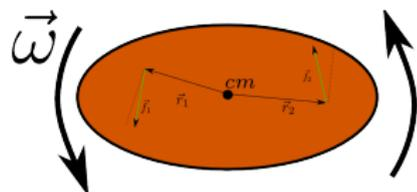
$$\begin{aligned} \frac{d\vec{P}}{dt} &= \sum_i \vec{f}_i & \vec{P}_{cm} &= m\vec{v}_{cm} \\ \frac{d\vec{L}}{dt} &= \sum_i \vec{\mathcal{T}}_i & \vec{L} &= I\vec{\omega} \\ \vec{\mathcal{T}}_i &= \vec{r}_i \times \vec{f}_i \end{aligned}$$
