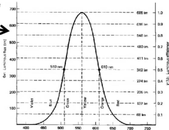
**Figure 2-7** CIE luminous efficiency curve. The luminous flux corresponding to 1 W of radiant power at any wavelength is given by the product of 683 lm and the luminous efficiency at the same wavelength:  $\Phi_v(\lambda) = 683V(\lambda)$  for each watt of radiant power.
