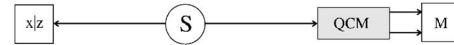
FIG. 1. Setup devised by Herbert to achieve signaling. A source S produces pairs of qubits in a maximally entangled state; on the left, Alice measures either \sigma_x or \sigma_z . On the right, Bob applies a perfect quantum cloning machine (QCM) and then measures the two clones (the measurement M may be individual or collective).
