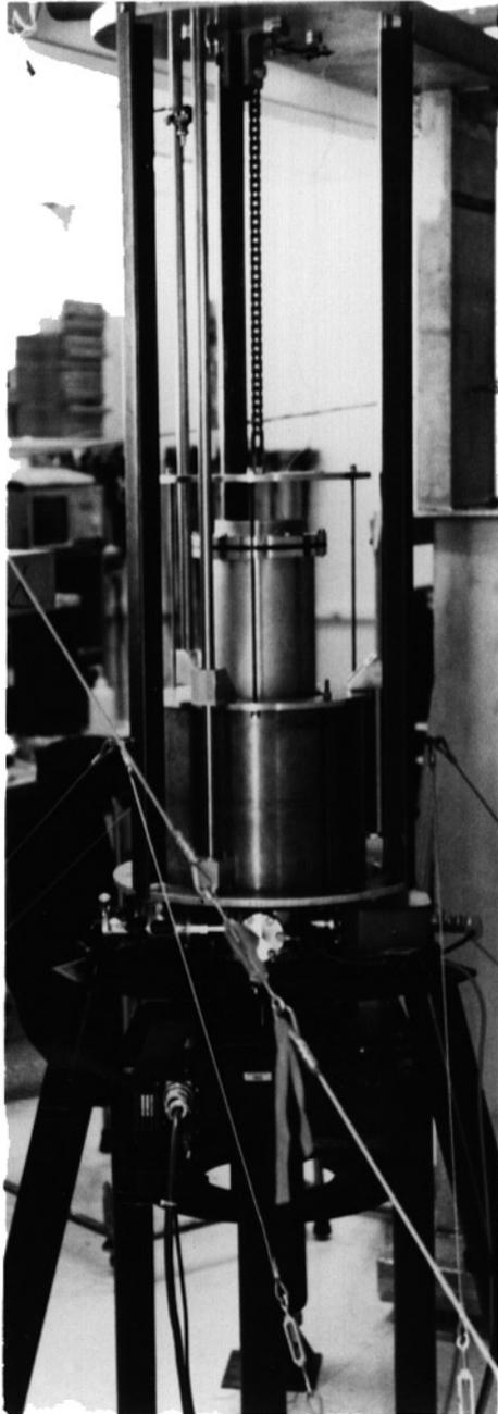
**Figure 9.** Photograph of the model FG5 absolute gravimeter and the moveable cylindrical source mass used to determine  $G$  at the Joint Institute for Laboratory Astrophysics in Boulder, Colorado, USA. The source mass is shown positioned around the dropping chamber of the gravimeter (courtesy of J E Faller).
