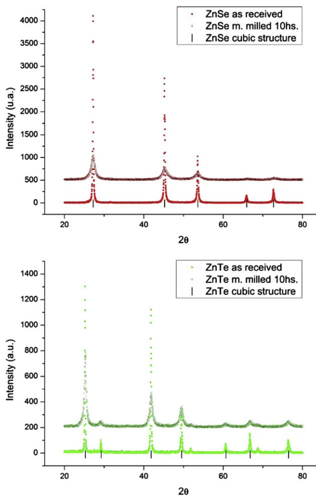
**Fig. 1** – XRD patterns for ZnSe and ZnTe powders as received and after 10 h of mechanical milling. (top) ZnSe as received and after 10 h of milling; (bottom) ZnTe as received and after 10 h of milling.
