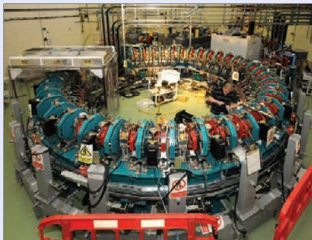
Round and round The EMMA proof-of-principle prototype accelerator can now store a particle beam.
